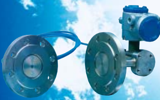
Closed tank level measurement. Seals DN80 / PN40, with capillary on HP side and rigid mounting on LP side.
