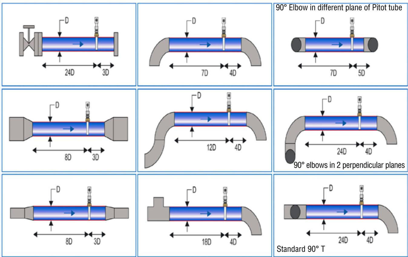
Chosen location for 5RD Pitot tube series set up in piping systems really matters because of the turbulence (secondary flow) in the flow created by the pipe configuration which can compromise the measurement accuracy. If the 5RD Pitot tube series is set up on shorter distance than advised, accuracy might be compromised but measurement repeatability will remain exact.
