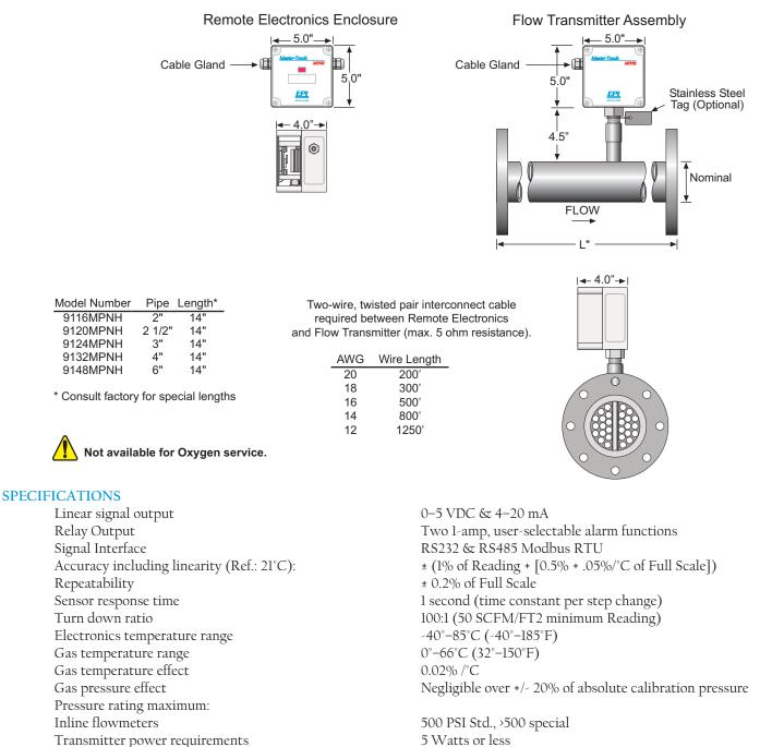
Pressure rating maximum: Inline flowmeters Transmitter power requirements RAM Back-up Wetted materials: Standard temperature & pressure (STP) (Air .075 lb/cubic foot) NIST traceable calibration
